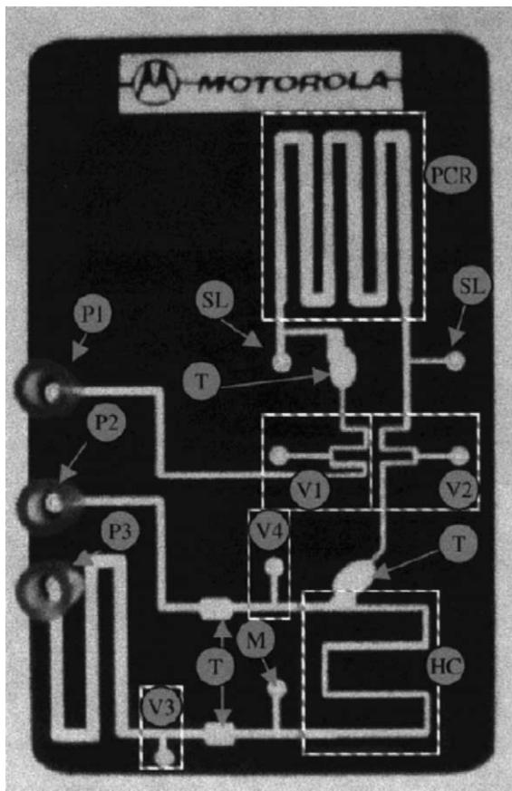
Fig. 2. Monolithic integrated polycarbonate DNA assay device. Serpentine PCR channel (PCR), hybridization channel (HC), Pluronic valves (V1–V4), Pluronic traps (T), hydrophobic air-permeable membrane (M), PCR reagent loading holes (SL), sample driving syringe pump P1, waste-withdrawing syringe pump (P2), and wash syringe pump (P3). Reprinted from [48] with permission.
