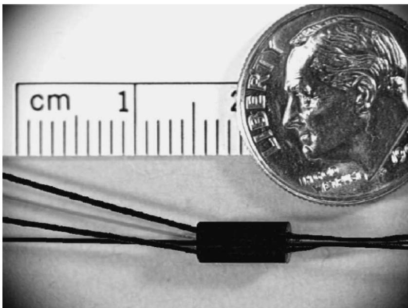
Fig. 5. Integrated fuel processor system, intended for use with a micro-fuel cell with an eye on providing power to remote electronic devices. The assembly consists of two vaporizer/preheaters, a heat exchanger, a combustor, and a steam reformer. Reprinted from [194] with permission. The work for this device was done by the Battelle Memorial Institute, Pacific Northwest Division.
