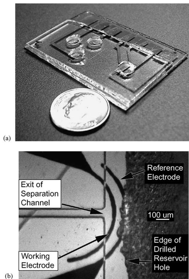
Fig. 3. (a) Photograph of a glass CE/EC microchip with integrated electrochemical detection and high voltage electrodes, designed for use with a portable system. The use of microfabrication techniques to integrate permanent electrodes into the chip minimizes the number of manual operations required for operation and reduces difficulties associated with variability in electrode placement and geometry. (b) Magnified top view of EC detection cell and electrodes. Reprinted from [77] with permission.
